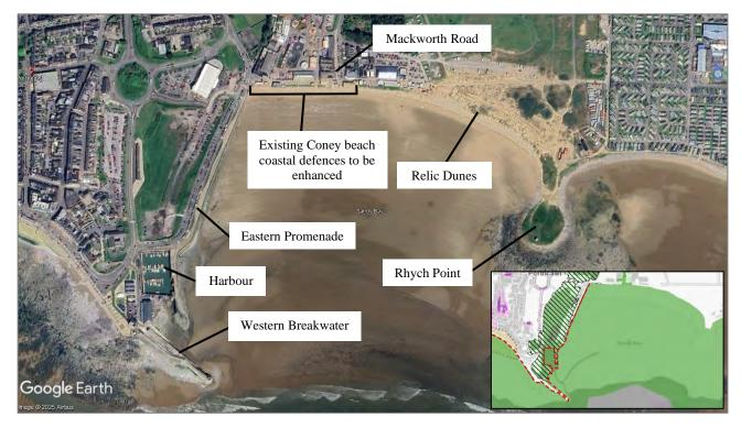
Figure 1: Location of key features within Sandy Bay. Inset image shows extract for Flood Map for Planning<sup>3</sup> with red dashed line indicating Flood Defences.
